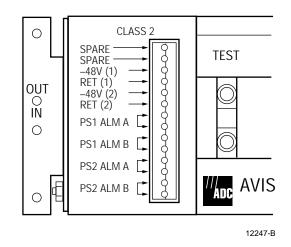
Figure 8. Power and Alarm Contacts
